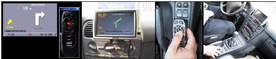
Image1: a sample screen of an interactive prototype based on the PC, and the VDO Dayton MS5000 system, as it was finally produced.
