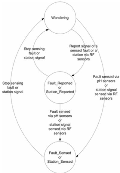
**Figure 4: Indirect communication protocol state diagram**
